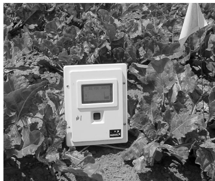
An irrigation monitor box collects water penetration data.
